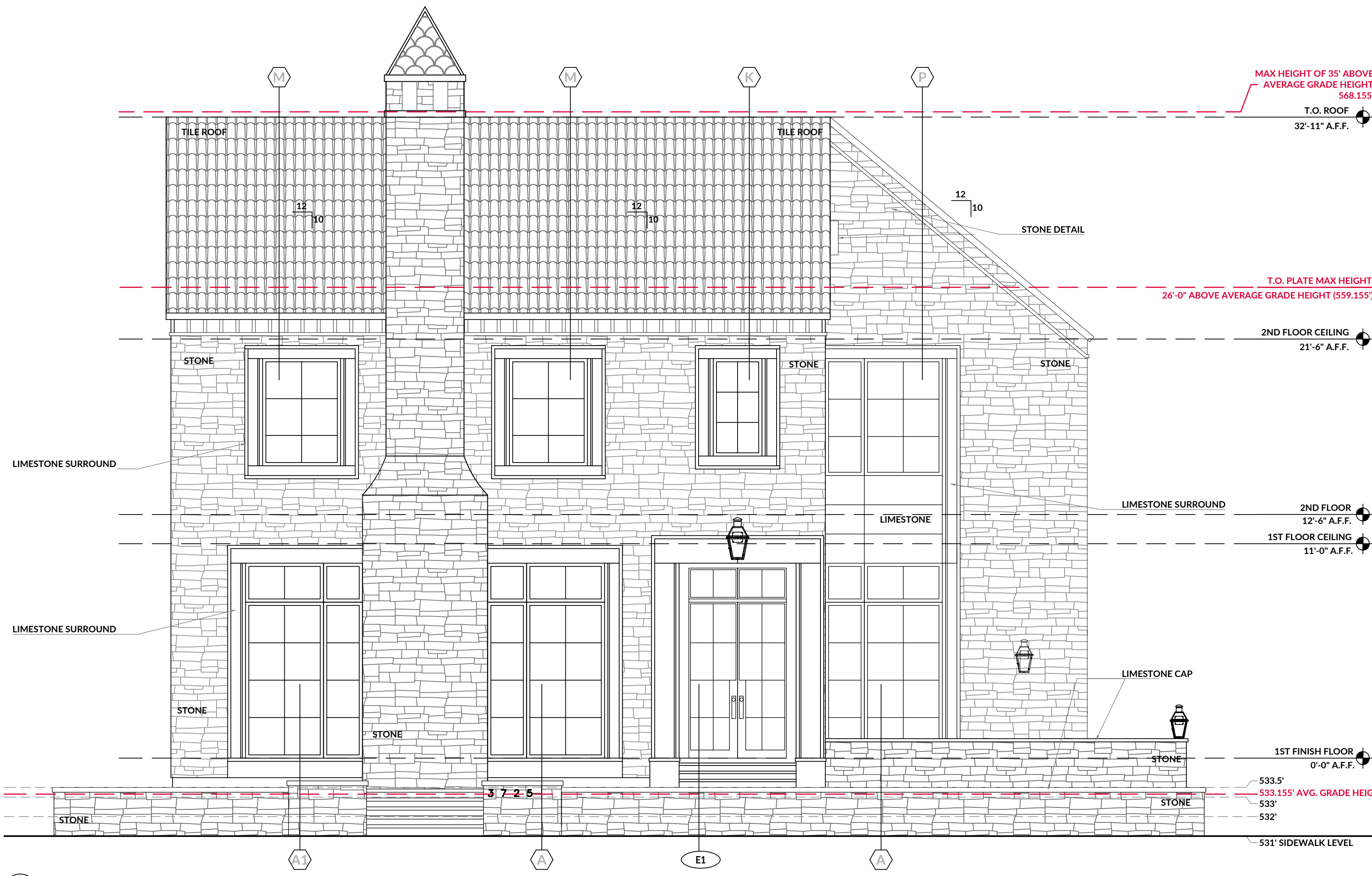
1 EXTERIOR ELEVATIONS | NORTH VIEW SCALE: 0' - 1/4" = 1' - 0"
